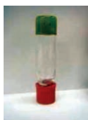
Figure 1. Quartz vial containing gel resulting from ROMP of DCPD using pre-catalyst 2a and PAG 3 .
